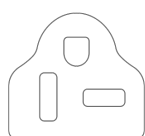
Power cord with plug (NEMA 6-20P)
