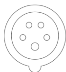
Power cord with plug (IEC 60309, 5-pol, CEE, red, 16 A)
